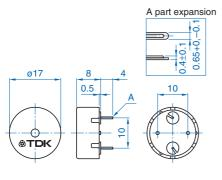
Tolerance:  $\pm 0.3$  Dimensions in mm
