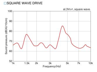
\* The frequency characteristic changes depending on the case shape and the installation method.
