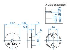
Tolerance: ±0.3 Dimensions in mm
