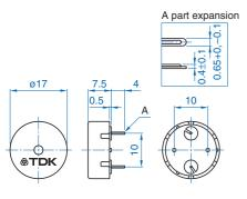
Tolerance:  $\pm 0.3$  Dimensions in mm
